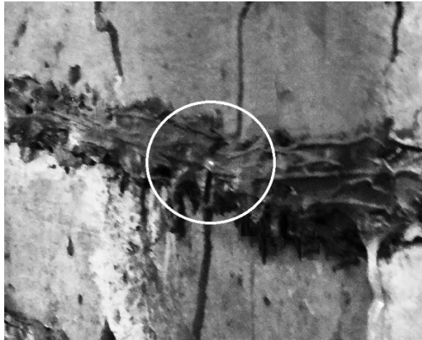
Fig. 1. The fracture and glow of the optical fiber, fixed with epoxy adhesive on a brick wall, due to the appearance of a crack in it (photo).
