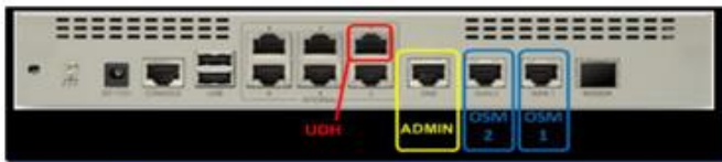
Figure 1: S3C - Fortigate 80c interface Panel (Two OSMs or RSG)
