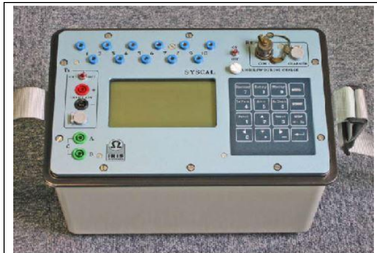
Fig. 18: Resistivímetro Syscal-Pro Switch 48 de Iris Instruments.
