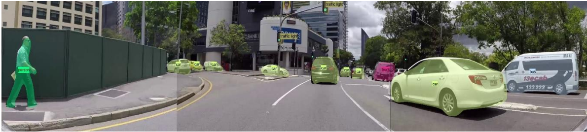
Figure 101.- Instance segmentation with Mask-RCNN.
