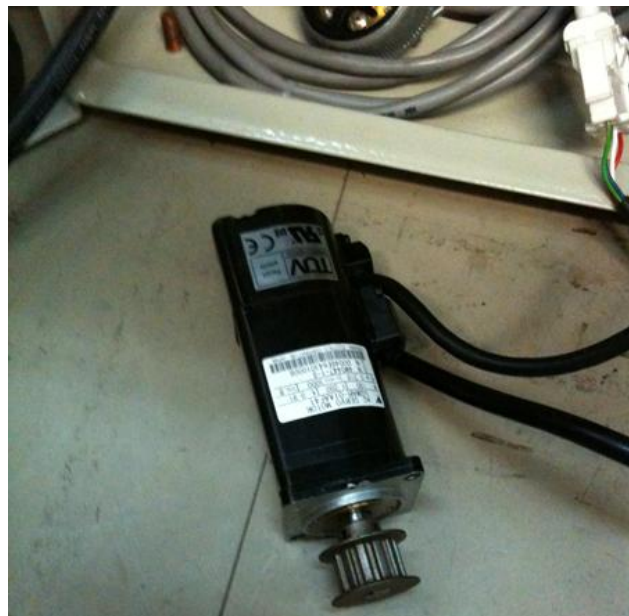
Figura 2.16. Servomotor SGMAH 01AAF.
