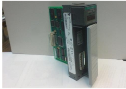
Figura 2.8. 1747-SDN Scanner DeviceNet®.
