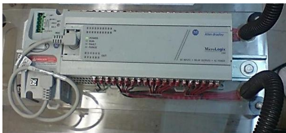
Figura 2.9 Micrologix 1000 Series E.
