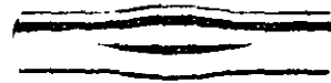
TYPE 5 — Center groove. Ideal for rod assemblies, also as a hinge pin.
