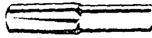
TYPE 4 — Half-length reverse taper. A variation of type 2 for use in blind holes.
