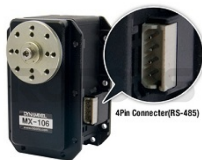
Figura 4.3: Servomotor dynamixel modelo MX-106.
