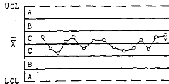
FIGURE 1. Illustrations of Tests for Special Causes Applied to Shewhart Control Charts
