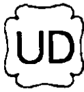
FIG. UG-129.2 OFFICIAL SYMBOL FOR STAMP TO DENOTE THE AMERICAN SOCIETY OF MECHANICAL ENGINEERS' STANDARD FOR RUPTURE DISK DEVICES
