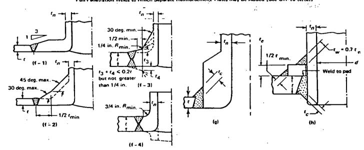
FIG. UW-16.1 SOME ACCEPTABLE TYPES OF WELDED NOZZLES AND OTHER CONNECTIONS TO SHELLS, DRUMS, AND HEADERS
