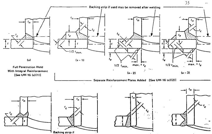
Full Penetration Welds to Which Separate Reinforcement Plates May be Added [See UW-16 (c)(2)]
