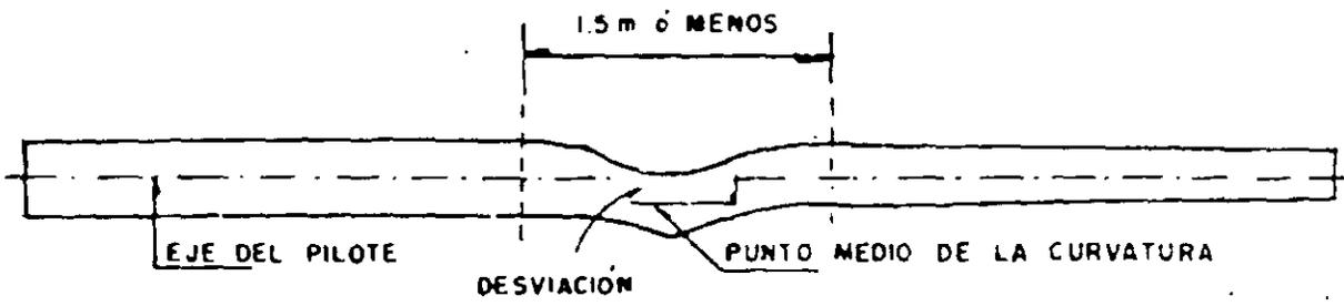
CASO 2. - LOS EJES DE LA SECCION ABAJO Y ARRIBA DE LA CURVATURA COINCIDE O SON PRACTICAMENTE COLINEALES
