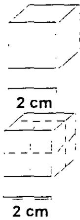
$$\begin{aligned} \text{área exp.} &= 2 \times 2 \times 6 = 24 \text{ cm}^2 \\ \text{masa} &= 8 \times 3 = 24\text{g} \quad \text{SEsp} = 1\text{cm}^2/\text{g} \end{aligned}$$
