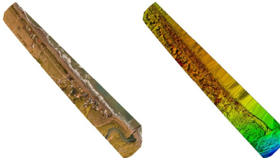
Figure 1: Orthomosaic and the corresponding sparse Digital Surface Model (DSM) before densification.
