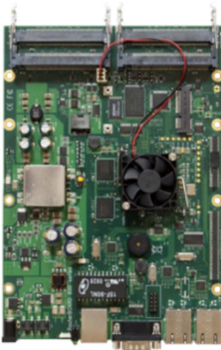
The RB800 is an advanced high performance wireless platform. It has four miniPCI slots, three Gigabit ethernet ports, two daughterboard connectors, a miniPCI-e slot and a compact flash slot.
