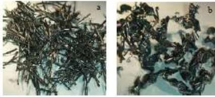
Fig. 16. Chip formation (a) High speed; (b) True spiral.
