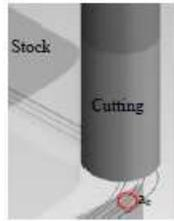
Fig. 4. Working engagement in contour operation – HSD.
