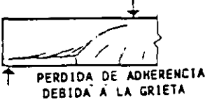
(a) SHEAR - TENSION FAILURE
