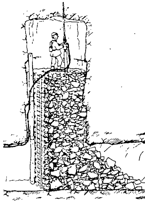
Fig. 7.25 Timbered raise shaft.
