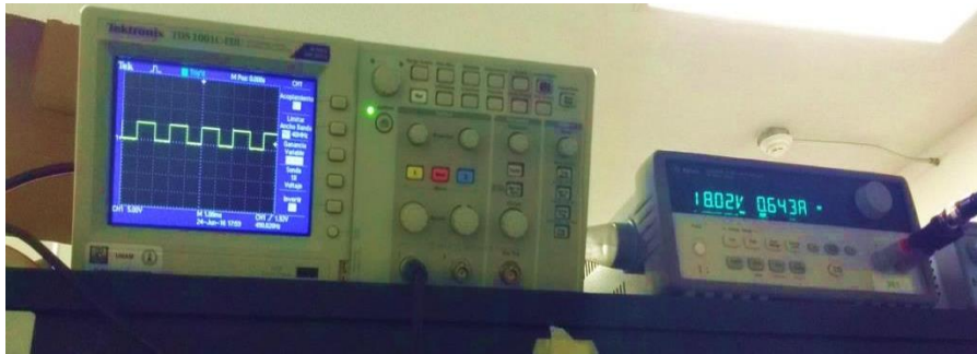
Figura 7.1.15 PWM 80% corriente de 0.643A
