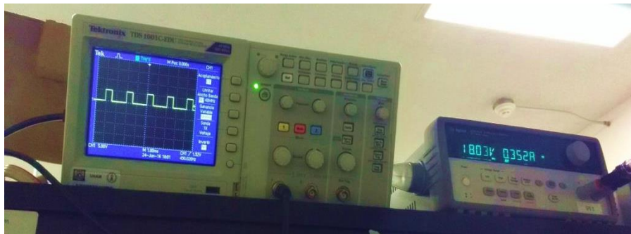
Figura 7.1.16 PWM 35% corriente de 0.352A
