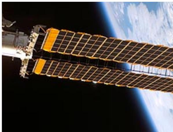
**Fig. 21 Arreglo de paneles fotovoltaicos de la estación espacial internacional.** Fuente: [https://www.nasa.gov/mission\\_pages/station/structure/elements/solar\\_arrays.html#.VvjB6JPhCRs](https://www.nasa.gov/mission_pages/station/structure/elements/solar_arrays.html#.VvjB6JPhCRs)
