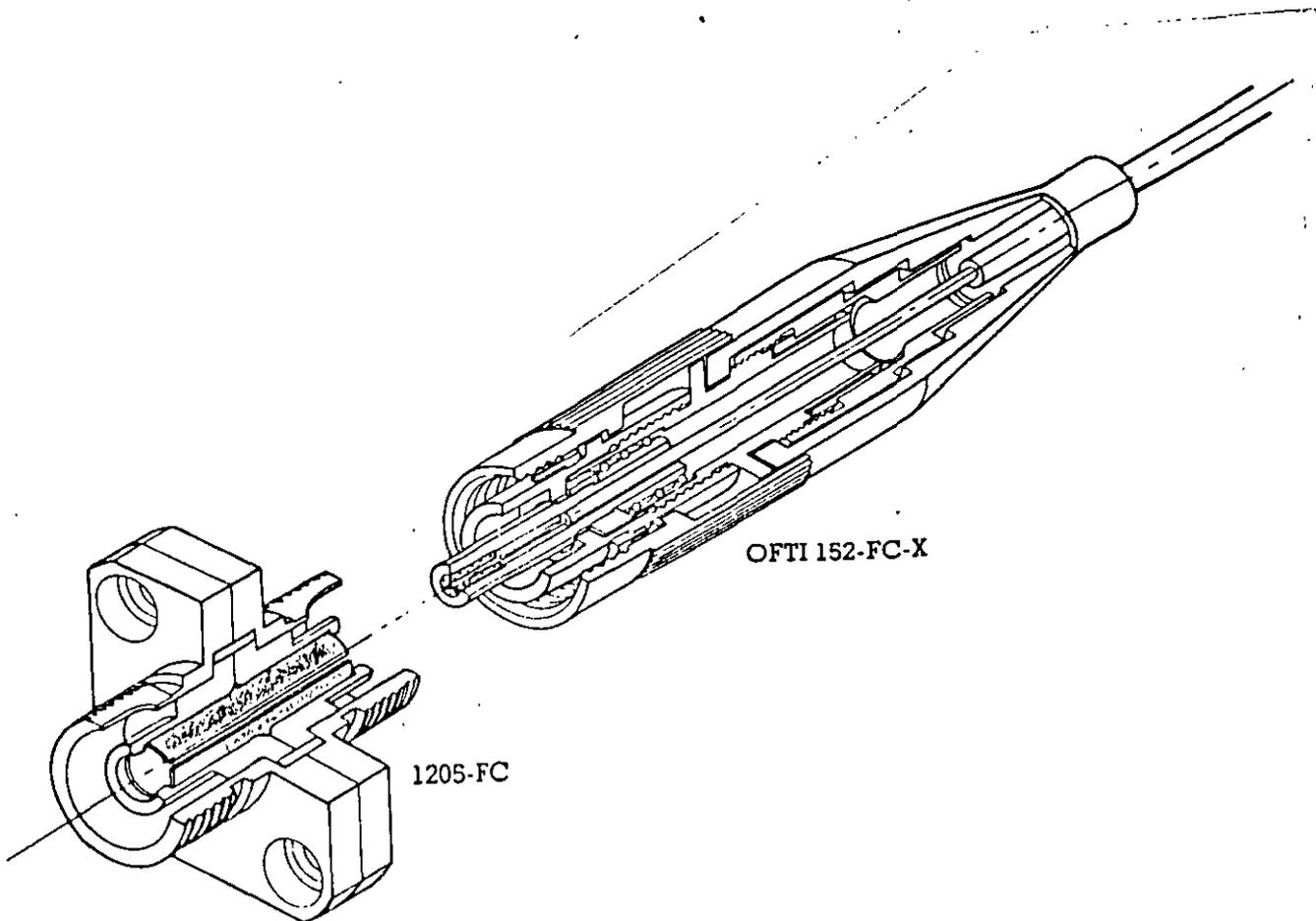
Fig.6 Corte transversal. Conector FC y cople.
