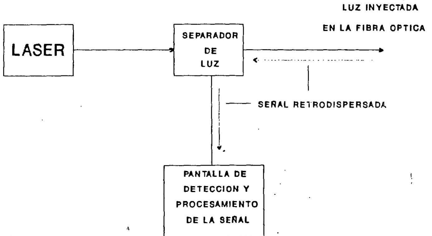
FIG. 8.20 PRINCIPIO BASICO DEL REFLECTOMETRO.
