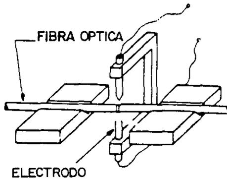
**FIG. 7.13 FUSION DE LA FIBRA POR ARCO ELECTRICO**
