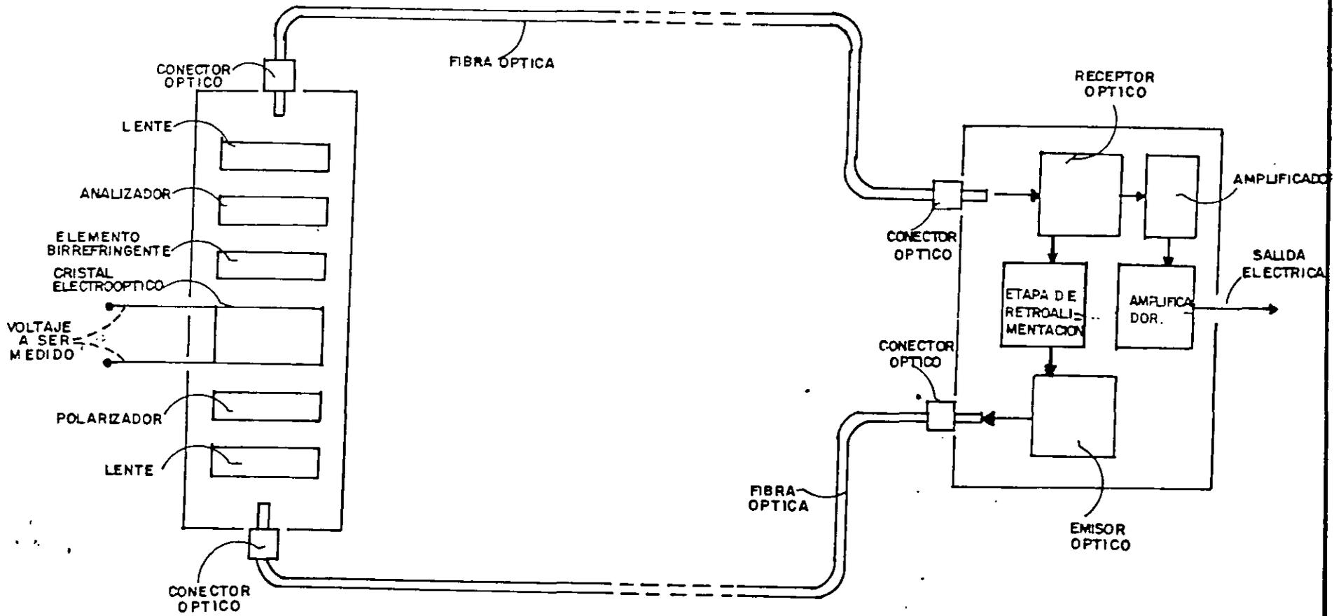
FIG. 4.1 DIAGRAMA A BLOQUES DEL SENSOR DE VOLTAJE.
