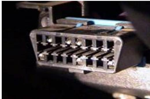
**Figura V.73 Conector DTC OBDII (Diagnostic Trouble Code) Consult II.**
