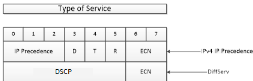
Figura 2.9. Campo Type of Service/DSCP.
