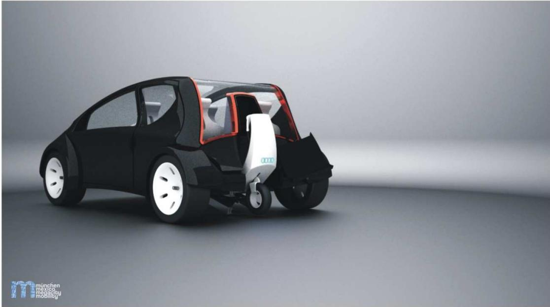
as soon as the front wheel contacts the ground, a linear gear pushes the scooter out to bring it into a perfect position
