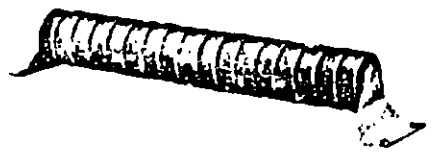
FIGURE 4.12 Flat belt rubber cushion impact idler, with fixed shaft
