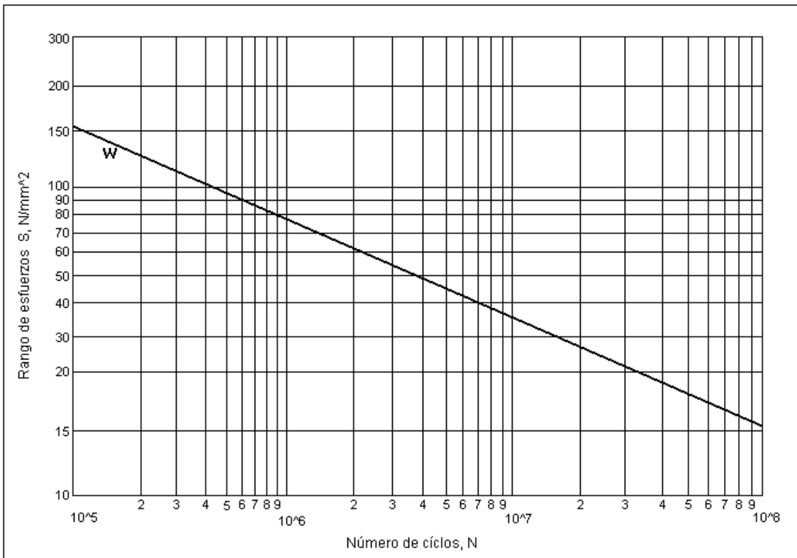
Fig. 2.23 Curva S-N (W) de la figura 2.22. Ref. [ 30 ]
