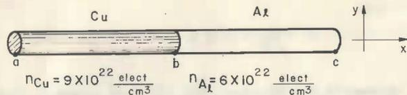
$$n_{Cu} = 9 \times 10^{22} \frac{\text{elect}}{\text{cm}^3} \quad n_{Al} = 6 \times 10^{22} \frac{\text{elect}}{\text{cm}^3}$$
