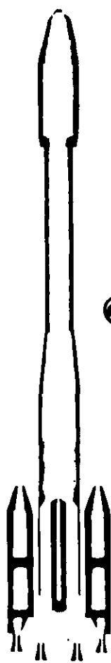
AR 44LP 2 solid strap-on boosters + 2 liquid strap-on boosters
