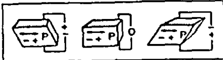
Figure 3. It is possible to produce various stresses and strains in the material by means of different combinations of the orientation of the crystal and the direction of the applied field. In this example, a field applied parallel to the piezoelectric axis produces elongation in the direction of the axis
