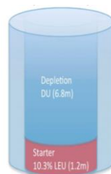
FIGURE 3.12. Conceptual drawing of CANDLE (Kim & Taiwo, 2010).
