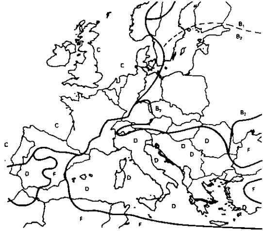
Figure 6.11-19 Rain rate climate regions for Europe. (From NASA Propagation Effects Handbook for Satellite System Design, ORI TR 1679.)
